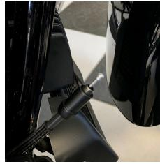
36. Slide the tube extension over the wire.
