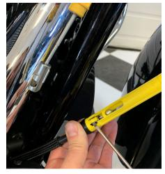
35. Use the two wrenches to loosen the adjustor on the wire extension. Slip the wire extension over the wire, hand tighten the nuts, bring the adjustor nut down, then tighten with the wrenches.
