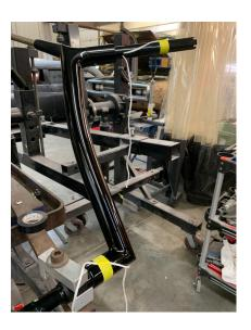
13. Installing the original handlebar control wires back into the bars. Start by taping the right control wire at the bottom side of the handlebar next to knurling. Pull right side rope up until wire comes out of grip tube. Then proceed with same procedure for left side.
