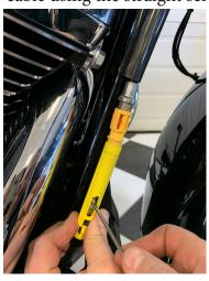
32.. Remove the yellow plastic piece by spreading open the two small tabs on each side.
