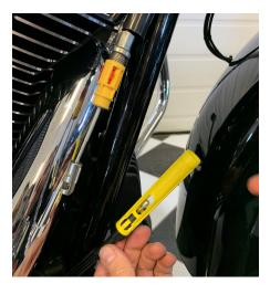
34. Remove the lower portion from the tube extension, and slide it over the stock cable.
