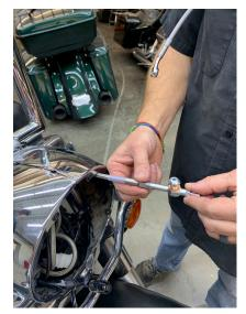
20. Attach stock clutch line to new bleeder fitting.
