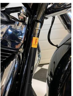
40. After you slide the cover back on, reinstall the frame clips.
