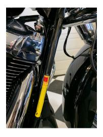
30. Push the wire through from the backside using the screwdriver.
