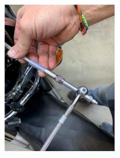
21. Pull brake line assembly into headlamp housing and attach to clutch master cylinder. Tighten all fittings.
