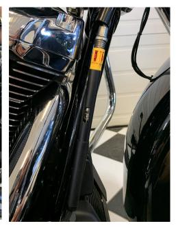
39. Now you can adjust the clutch cable and reinstall the black tube cover.
