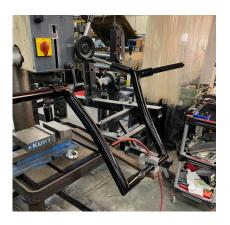
11. Using supplied ropes and air blower, push 2 ropes through the right FBI handlebar grip tube and bring through center clamp hole. Push 1 rope through left FBI handlebar grip tube and bring through center clamp hole.
