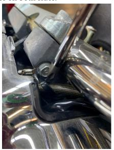
8. Unplug left hand switch housings and throttle sensor plugs and remove stock handlebars.
