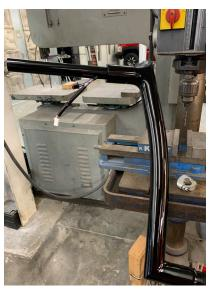
15. Pull throttle wires through the right handlebars from the grip tube down through the hole in the clamp area as normal. Note: Make sure control wire is installed first.
