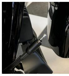
29. Rotate the yellow tube, and locate the little tab. Then separate it from the lower cable using the straight screwdriver.
