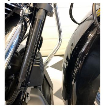
2. Remove the cable clips from the frame. They will be reused.
