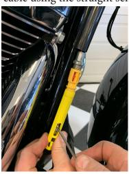
8. Remove the yellow plastic piece by spreading open the two small tabs on each side.
