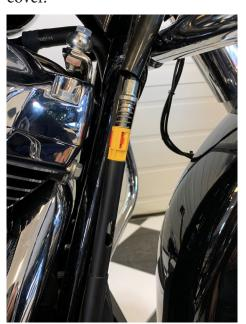
16. After you slide the cover back on, reinstall the frame clips.
