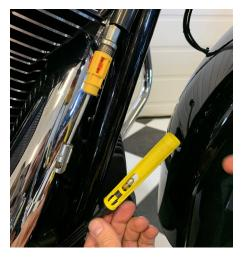
10. Remove the lower portion from the tube extension, and slide it over the stock cable.
