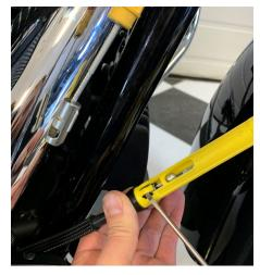
11. Use the two wrenches to loosen the adjustor on the wire extension. Slip the wire extension over the wire, hand tighten the nuts, bring the adjustor nut down, then tighten with the wrenches.
