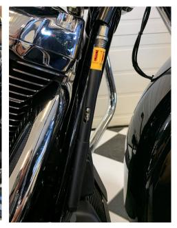
15. Now you can adjust the clutch cable and reinstall the black tube cover.
