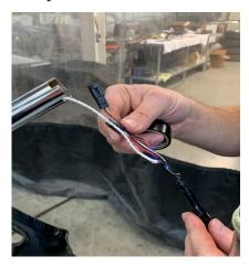
21. Tape right switch housing wires to the left string that comes out the grip housing hole.
