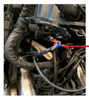
Stock handlebar throttle wire location
