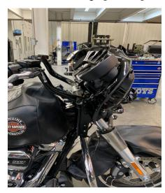
11. Cut the 2 zip ties on the handlebar risers that hold the brake and clutch line. Cut 1 zip tie that holds the clutch and brake line together.
