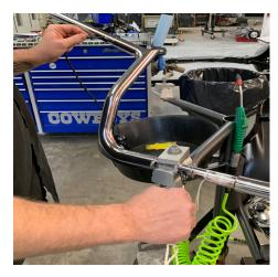
19. Some early models have a large, 6-wire molex throttle wire plug which will need removed and reassembled. Write down the wire color to corresponding terminal for reassembly of the plug. Grab the center holes with needle nose pliers and pull white center until a click is heard. Insert a paper clip into the small hole next to the wire pin to release all the wires.
