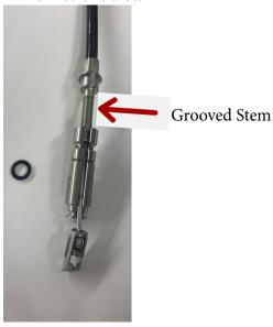
Note\*\*If your grooved stem is broken, make sure that the grooved stem is inside of the new adjustor when installing\*\*
