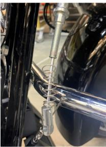
4. The photo below shows the parts that you are removing from the stock upper cable.
