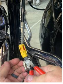
3. Now remove the spring by spreading open the end of the spring and twisting it off of the wire.
