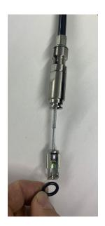
7. The new adjustor should look like the picture below when installed. After adjusting the clutch, tighten the locking nut.
