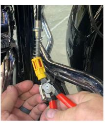
3. Now remove the spring by spreading open the end of the spring and twisting it off of the wire.
