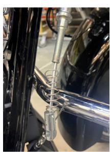
4. The photo below shows the parts that you are removing from the stock upper cable. This yellow adjustor is from a 2021 Model bike. If you have a 2022-2023 model, this piece is black.
