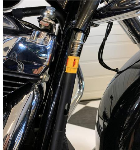
16. After you slide the cover back on, reinstall the frame clips.
