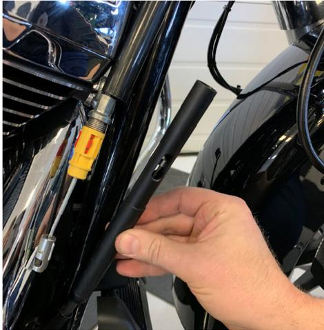
13. Push the upper clutch cable up the frame, and reinstall into the new clutch extension tube.
