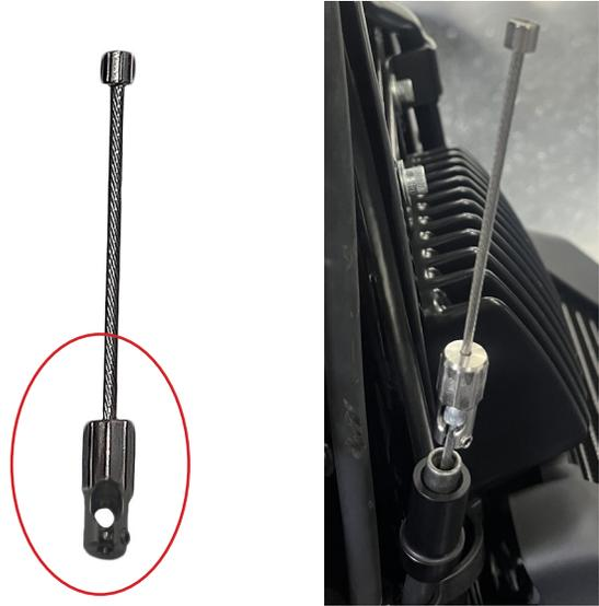
12. Slide the tube extension over the wire.
