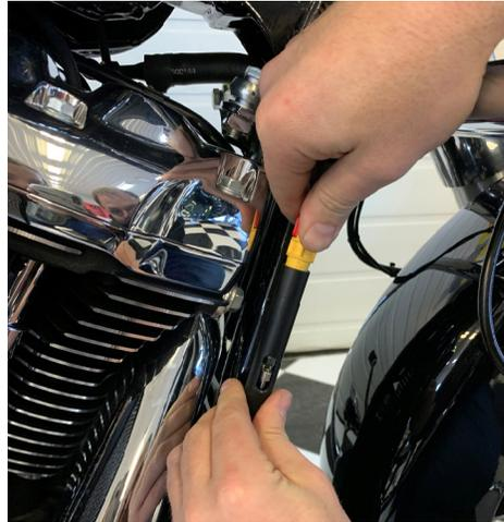
14. Connect the upper cable to the lower cable, through the oval opening in the black tube.
