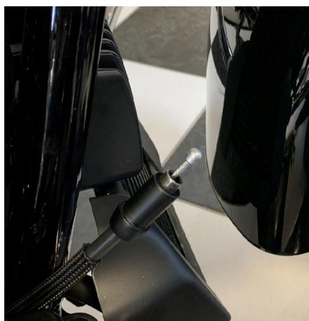
11a. If you have a clutch extension wire like the one in this picture below. Use the two wrenches to loosen the adjuster on the wire extension. Slip the wire extension over the wire, hand tighten the nuts, bring the adjuster nut down, then tighten with the wrenches.
