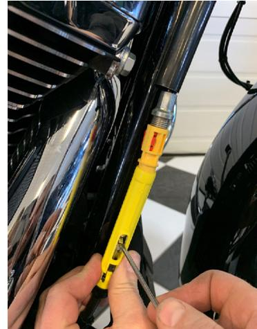
6. Push the wire through from the backside using the screwdriver.
