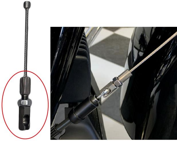
11b. If you have a clutch extension wire like the one in this picture below. Slip the wire extension over the wire, apply loctite to the set screw and use a 5/64 allen to tighten the set screw against the ball of the lower cable.
