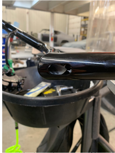
Access hole in bottom of handlebar.
