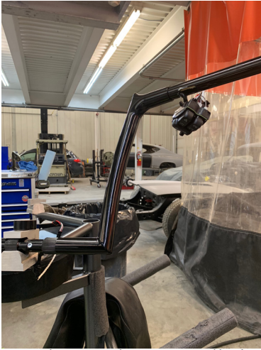
Right switch wires pulled through right handlebar.
