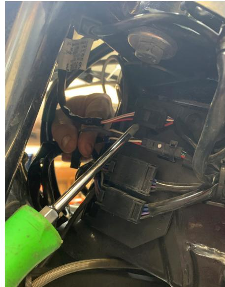
9. Install center handlebar bolt. Torque to 10 ft. lbs.
