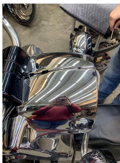
5. Remove the 3 screws that hold down the handlebar clamp cover and remove.
