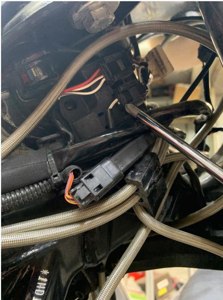
8. Unplug left hand switch housings and throttle sensor plugs and remove stock handlebars.
