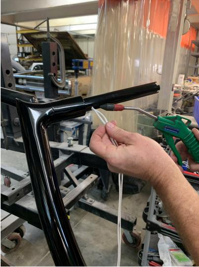
12. Tape 1 string out of the right handlebar to the right grip tube and lower clamping area. This will be used later to run throttle wires through handlebar.
