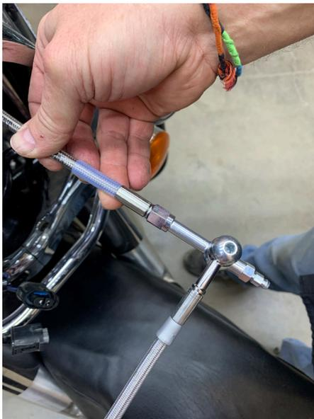
21. Pull brake line assembly into headlamp housing and attach to clutch master cylinder. Tighten all fittings.
