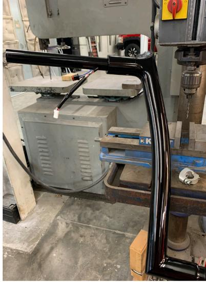
15. Pull throttle wires through the right handlebars from the grip tube down through the hole in the clamp area as normal. Note: Make sure control wire is installed first.
