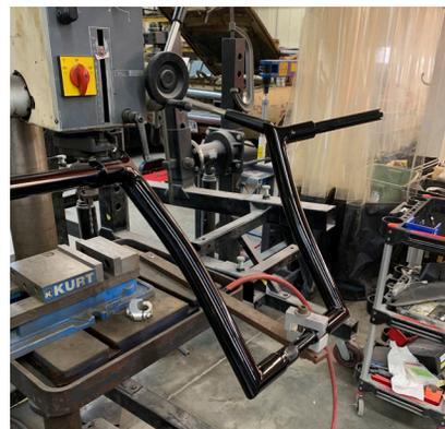
11. Using supplied ropes and air blower, push 2 ropes through the right FBI handlebar grip tube and bring through center clamp hole. Push 1 rope through left FBI handlebar grip tube and bring through center clamp hole.
