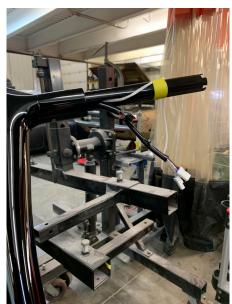
14. Tape left handlebar wires to the string at the clamp area of the left handlebar. Lubricate taped area and pull wires up through handlebar.
