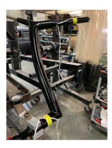
13. Installing the original handlebar control wires back into the bars. Start by taping the right control wire at the bottom side of the handlebar next to knurling. Pull right side rope up until wire comes out of grip tube. Then proceed with same procedure for left side.
