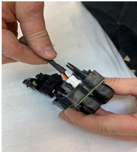
17. Take the left switch housing and tape wires to the left string at the grip housing hole. Apply supplied petroleum jelly to the wire loom.
