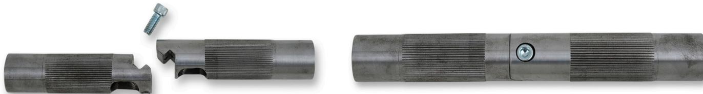
2. Using the supplied ropes, use an air blower to push 1 rope through the left handlebar grip tube hole to the center clamp hole. Next, blow the 2nd rope through the right handlebar grip tube hole to the center clamp hole. Then, blow the 3rd rope through the right handlebar throttle hole to the center clamp hole.
