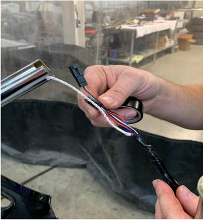
21. Tape right switch housing wires to the left string that comes out the grip housing hole.
