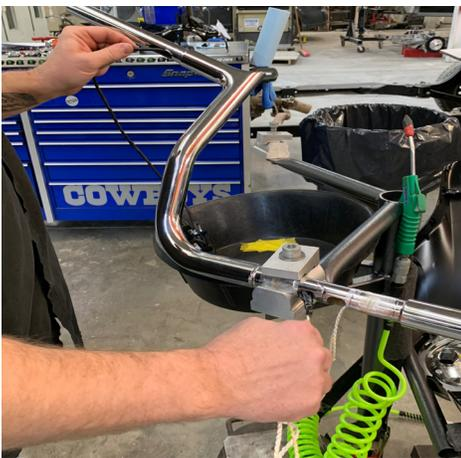
19. Some early models have a large, 6-wire moxex throttle wire plug which will need removed and reassembled. Write down the wire color to corresponding terminal for reassembly of the plug. Grab the center holes with needle nose pliers and pull white center until a click is heard. Insert a paper clip into the small hole next to the wire pin to release all the wires.
