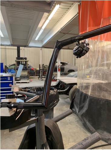
Right switch wires pulled through right handlebar.
